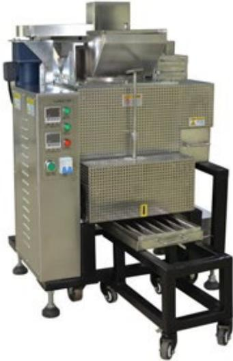
Solder dross separator SDS-10MS has Patent mixing and separation system which make separation more efficient and easier for operation, it is a best solution for small batch solder dross separation.
