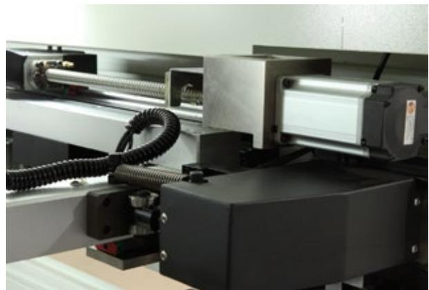
Servo-driven, closed-loop control blade system
