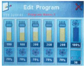
The easy to program on-board LCD with graphic user interface enables independent zone programming and maximum fl exibility in profile parameter control.
