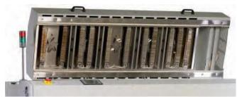
Plenum convection heating provides uniform temperature profiling across the entire PCB board.
