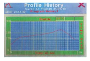
On-board LCD display provides graphical real time and historical program profiles.
