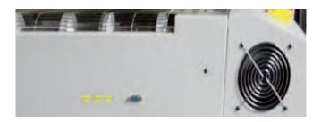
Attach three thermocouples for monitoring actual board temperature and download profile data and error logs via D9 connector.
