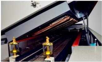
Conveyor: Chain and mesh belt conveyor,all rail has been harden-treated to stand the wear by chain, meanwhile standard equipped with lubrication cup.
