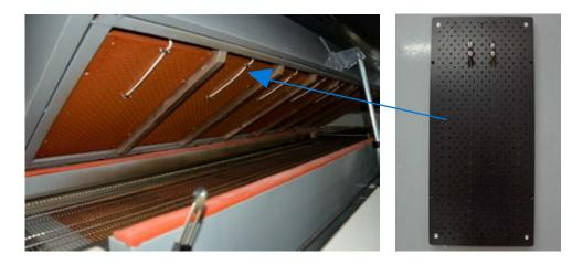
Latest self-designed porous plate, get best uniform hot air distribution under the theory of static pressure.New designing :aluminum heating plate +U shape heating tube, more stabile and longer service life.
