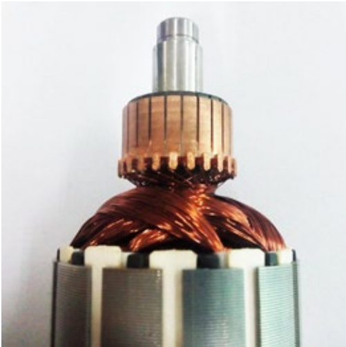
The motor rotor inside the enameled wire and the terminal of the welding, is the use of resistance spot welding.
