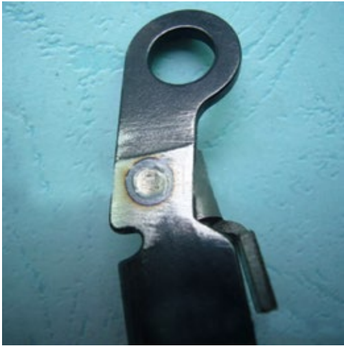
Copper, stainless steel pieces, and so are the hardware with a resistance spot welding.
