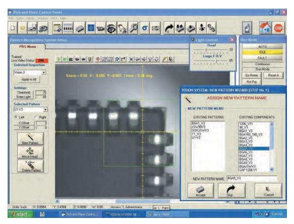
The vision software is Windows® based to allow easy straightforward teach-in, requiring minimal operator training.
