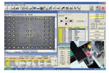
LS40V & LS60V vision assist pick & place systems use the full features of Cognex® vision centering. Bottom, top and on-the-fly places CSPs, micro BGAs and 15 mil pitch QFPs
