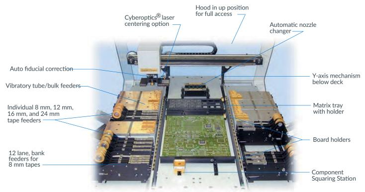
Model L60 showing easily accessible, unobstructed work deck
