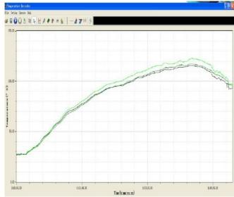
As for above profile, IR panel can get better uniform temperature than IR tube.
