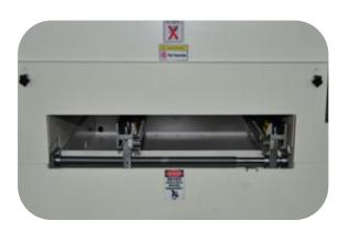
At entrance and exit there are plate we can adjust the height, so to prevent heat lose from both end.
