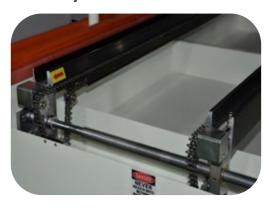
Stainless steel chain conveyor with harden guiding rails, 5MM pin length for conveyor chain.
