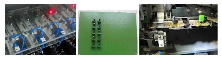
Tooling to accommodate a variety of applications-field reconfigurable Single Span: 2.5mm Dual Span: 2.5mm/5.0mm Triple Span: 2.5mm/5.0mm/7.5mm
