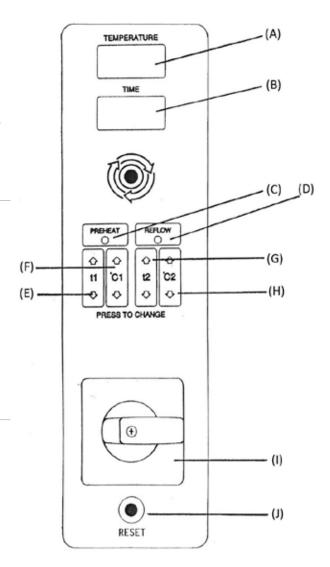
the status of the hot air heating. If the point lights on, heating is powered, and the temperature rises. The decimal point one digit to the left has the same function for the quartz heating.
