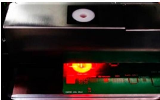
Uniform ring light and high brightness coaxial light ,equipped with ultra adjustable brightness control, makes all types of fiducial mark well recognizable (including rugged fiducial mark) and is applicable for all type of PCB and surface treatment. CCD can read incomplete or defective fiducial mark.
