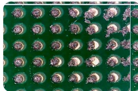
**Conclusion:** Printing result is perfect , no misalignment, shift, solder bridge, lack solder, etc.
