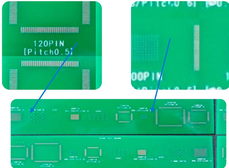
Use same sample to test H450 and other brand to check IC and BGA
