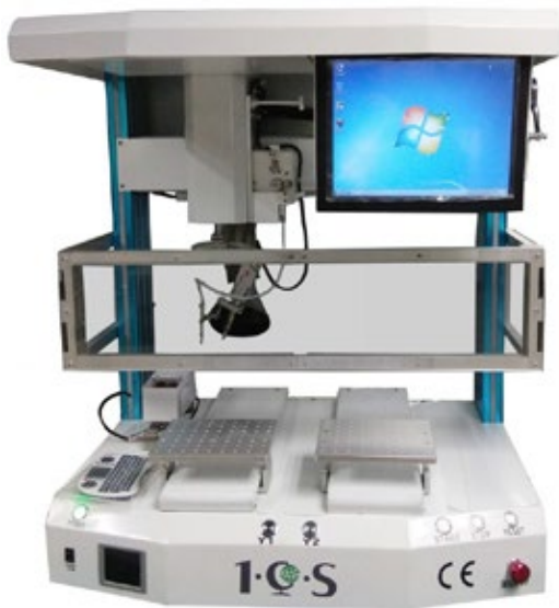
H352 Can handle PCBs up to 235x320mm*2PCBs
