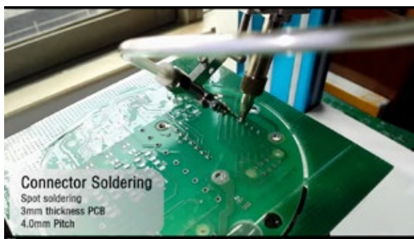
High heat soldering point(connector)
