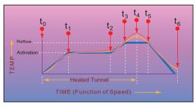
Theoretical Reflow Profile Typical Profile for Model 1200 (3 Vertical Heating Zones) Typical Reflow Profile for Model 2000 (7 Vertical Heating Zones)
