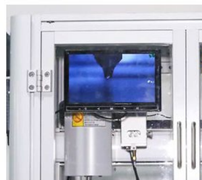
Vision options to monitor the soldering effect throughout the process, and can handle high-precision product soldering.
