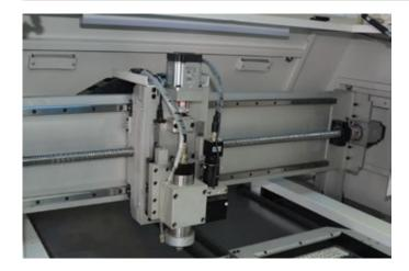
X,Y,Z axis adopt panasonic servo motor and it's driving system ,ball screw drive with rail & slider, make movement smoothly and precisely.
