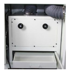
Built in 2.2KW vaccum cleaner provide a clean and low noise work environment.
