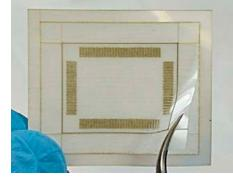
STEP 2 From the corner work the stencil off the backing material.
