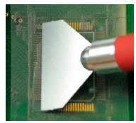
STEP 6 Inspect to make sure the "bumps" are uniform and consistent on all of the pads.
