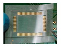
STEP 4 Finish aligning and placing the stencil.
