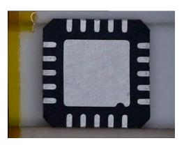
STEP 1 Remove device from PCB. Wick or scavenge and clean part.
