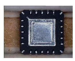
STEP 4 Remove StencillMate<sup>™</sup> from device clean and inspect.
