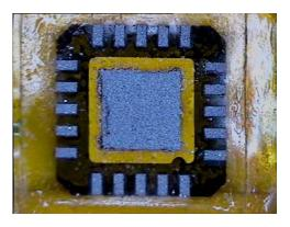
STEP 2 Place the part StencilMate <sup>™</sup> aligning it with part lands and applying pressure to the stencil. Squeegee solder paste with a manual squeegee into the apertures. Clean off surface of stencil.
