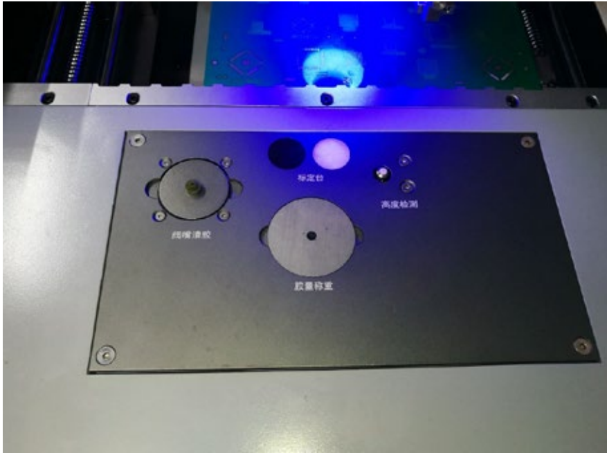
X/Y/Z correction platform. Nozzle suction cleaning. Glue weighing device (option).
